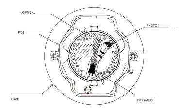
Fig.2 Top section, Series 27 Optical Smoke Detector
