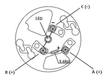
The MiniDisc Remote Indicator is polarity sensitive.
